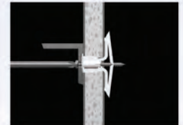
Place item over anchor and tighten until screw is flush with fixture. Then, stop.
